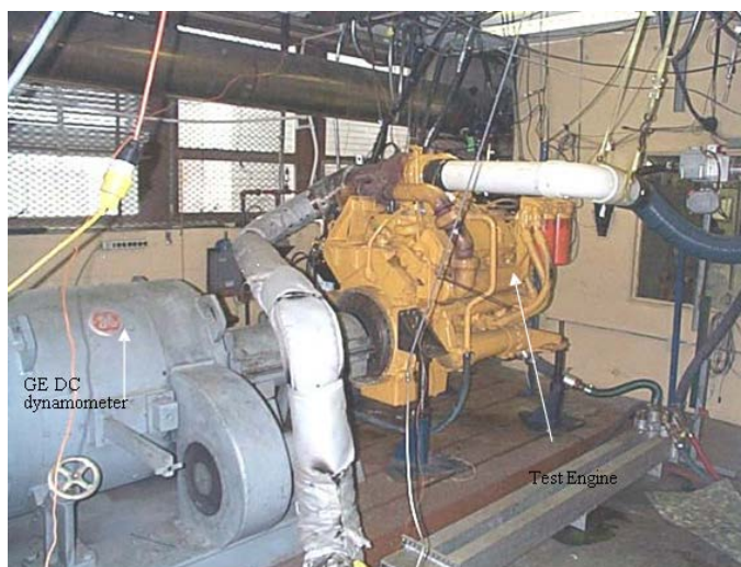
Fig. 6 Test engine coupled with GE DC dynamometer
