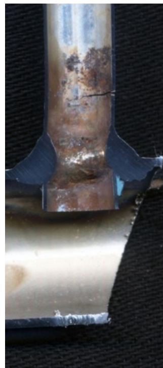
Figure 1 Macro photo of welded segment (branch weld) cut for metallographic preparation
