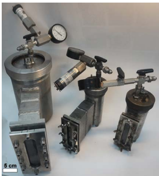
Fig. 1 Experimental set-up for combustion synthesis (stainless-steel reactors
